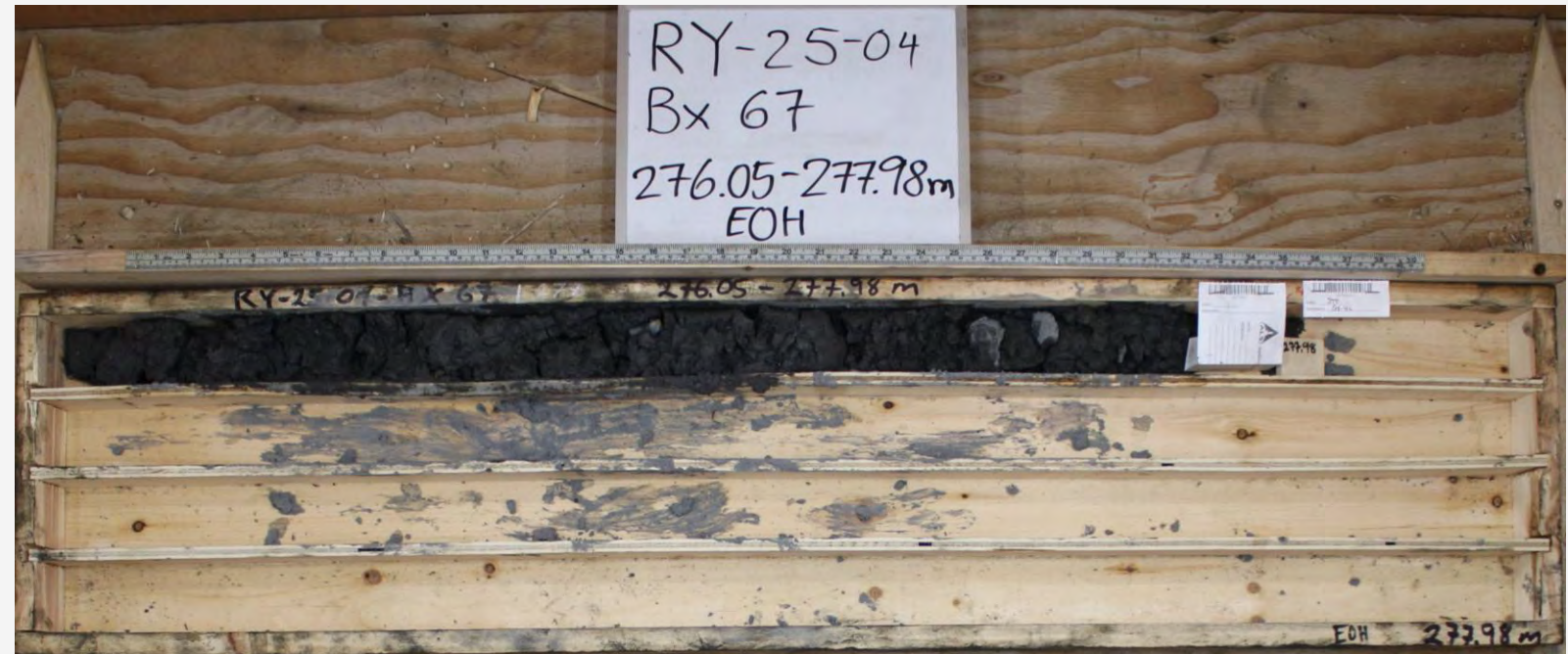
Drill core from hole RY-25-04, (276.05 m to 277.98 m) Fault gouge with high-grade silver
